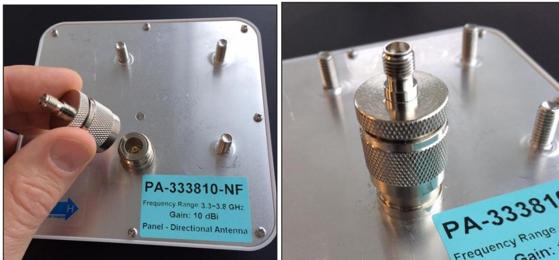
Figure 6—Connecting the SMA adapter to the antenna.
