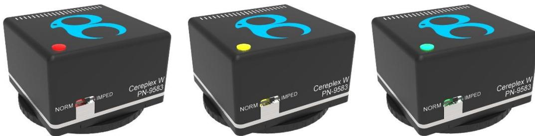
Figure 3 - The battery status indicator turns RED when the battery is low, YELLOW when it is charging, and GREEN when it is fully charged. The battery status LED is not illuminated while the headstage is in use and the battery is not low.
