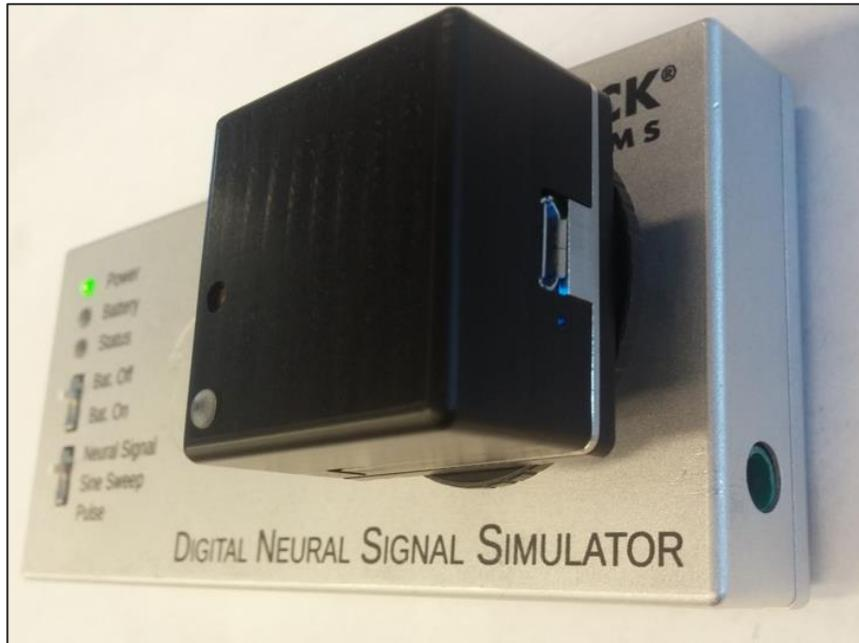
Figure 7—The CerePlex W headstage connected to the pedestal connector of the DNSS
